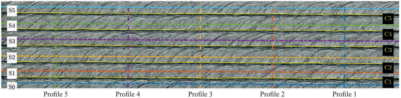
(c) Top view of milled aluminum cuboid block with steps S0-S5, edge contours C1-C5, and five surface profiles.
