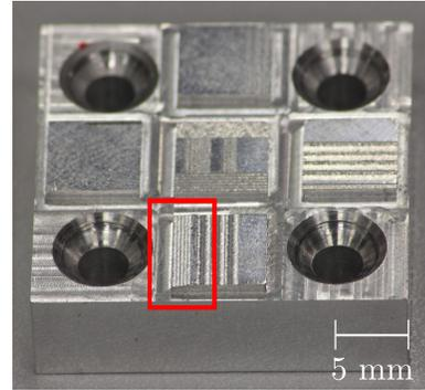
Fig. 5: Close-up view of aluminum block with holes for fixation and cuboids used for milling experiments. Area enclosed by the red box shows results of milling experiment from Sec. V-B.
