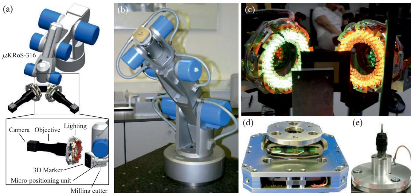
Fig. 1: Schematic of the macro-micro-manipulator setup (a) with its components: Macro-positioning unit  $\mu$ KRoS-316 (b), stereoscopic vision system (c), micro-positioning unit XYZ200M (d), and end-effector milling tool (e).
