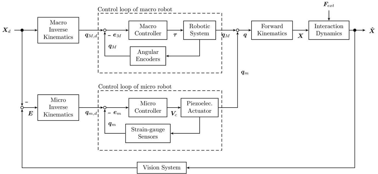
Fig. 4: Schematic block diagram of decoupled disturbance rejection design with vision feedback. External force  $F_{ext}$  and its interaction dynamics are unknown and compensated by visual feedback and micro-positioning unit. The corresponding coordinate transformations are omitted for the sake of clarity.
