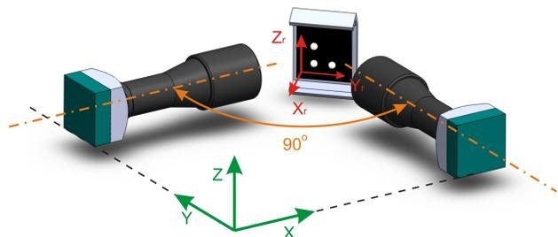
Fig. 2: Schematic for camera calibration system setup showing world frame (green) and reference frame of the 3D marker (red).
