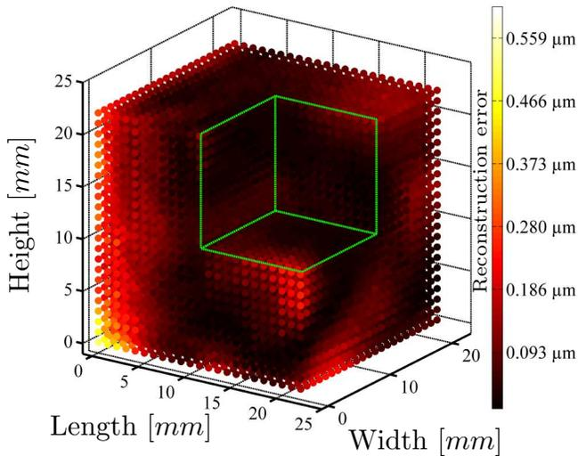
Fig. 3: Reconstruction error of calibration via essential matrix with light correction. Reference is provided by a coordinate-measuring machine.
