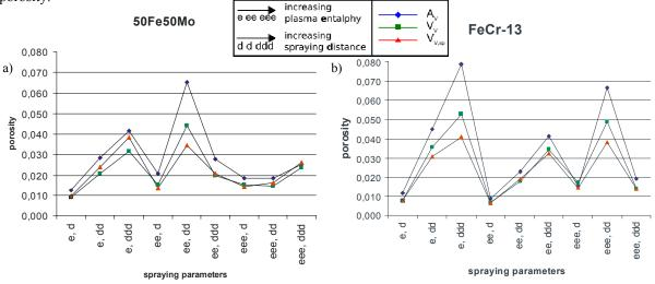
Fig. 4. different porosities made with different spraying parameters
