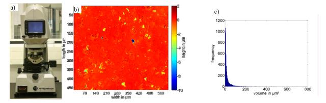
Fig.1 (a) measuring device white light interferometer; (b) measurements of the structures; (c) histogram of several measurements
