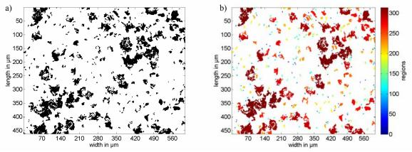
Fig. 3 (a) result of the watershed transformation of the measurement shown in Figure 1(b); (b) segmented regions
