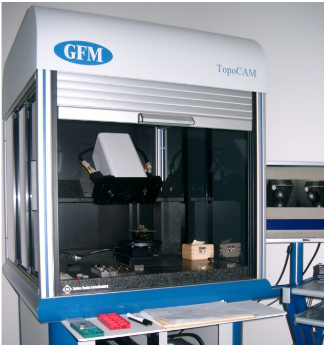
Fig. 2 Implementation of the optical 3D coordinate measurement machine TopoCAM
