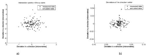
**Fig.2** Comparison of measured and simulated data - a) Deviation of the position vector (intersection point through the xy-plane):  $S_{m,x} = 0.54 \mu m$ ,  $S_{m,y} = 0.97 \mu m$ ,  $S_{sim,x} = 0.44 \mu m$ ,  $S_{sim,y} = 1.50 \mu m$  b) Deviation of the direction vector:  $S_{m,x} = 0.006 \mu m$ ,  $S_{m,y} = 0.011 \mu m$ ,  $S_{sim,x} = 0.019 \mu m$ ,  $S_{sim,y} = 0.005 \mu m$
