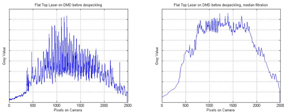
Figure 5 : Flat Top without rotating diffuser before (left) and after (right) median filtration
