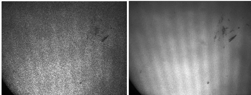
Figure 7 : Laser projected fringe pattern without (left) and with (right) rotating diffuser
