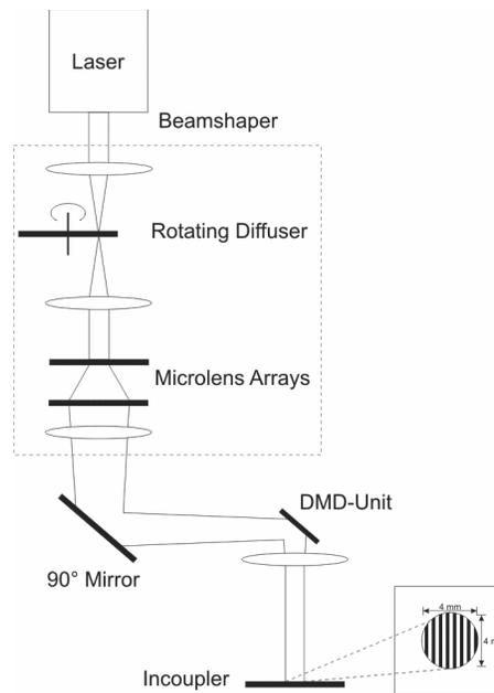
Figure 3 : Beamshaper setup (schematic)
