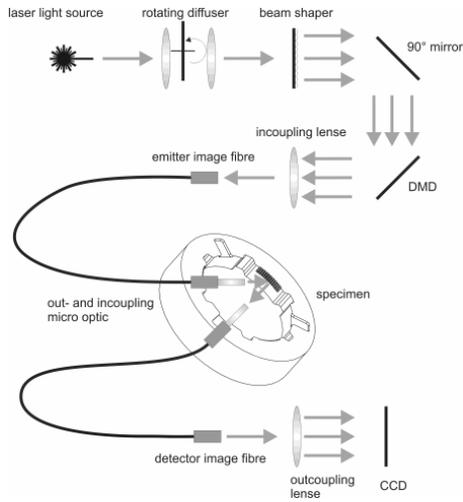
Figure 4 : Final setup (schematic)
