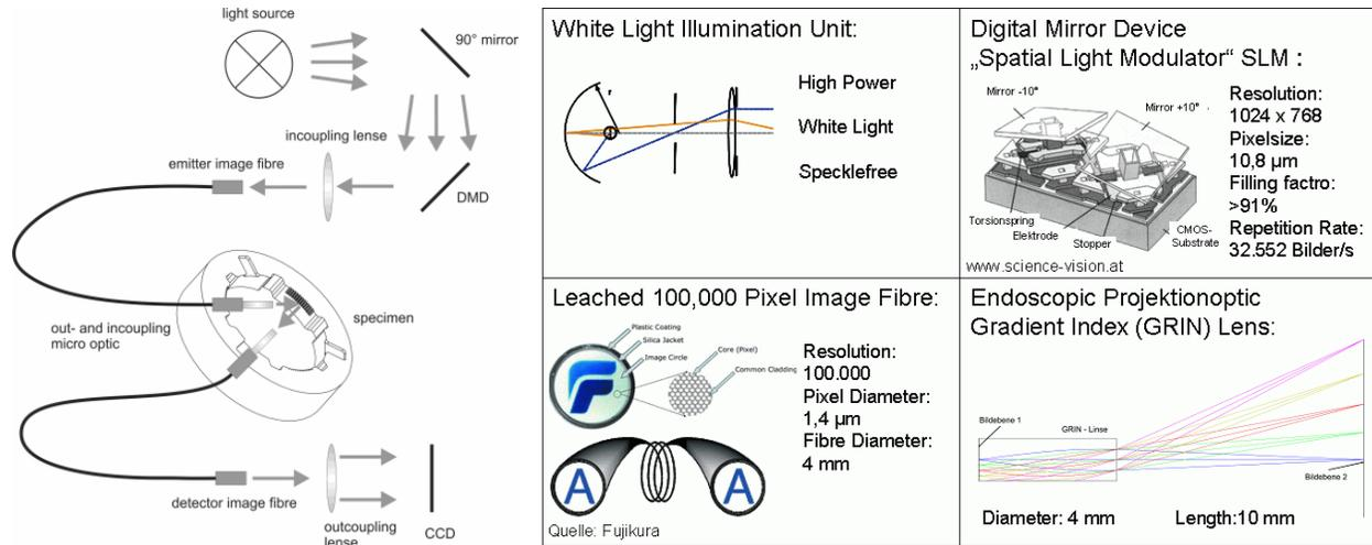
Figure 1: First approach setup (schematic) left; used components (right)
