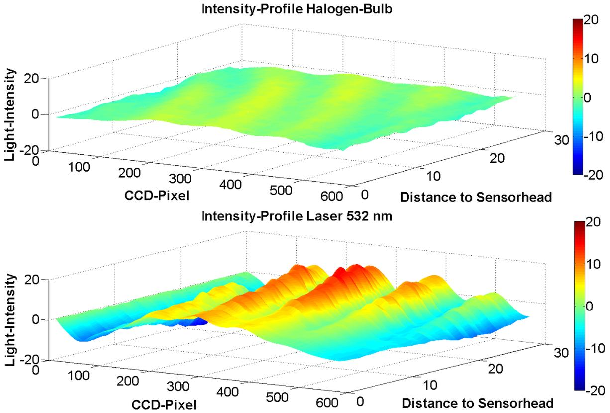
Figure 8 : Intensity distribution of a projected fringe pattern on the CCD-Camera with 150 W Halogen-Bulb (top) and Laser Illumination (bottom)
