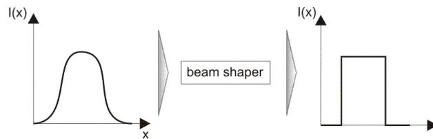
Figure 2 : Beam shaper intensity profile
