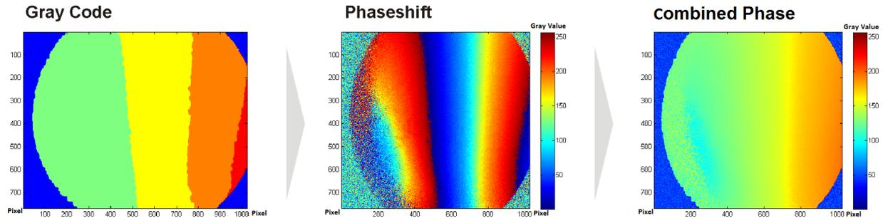
Figure 10 : Phase Algorithm on a flap surface (Grey Code – top, Phase shift – middle, combined phase - bottom)
