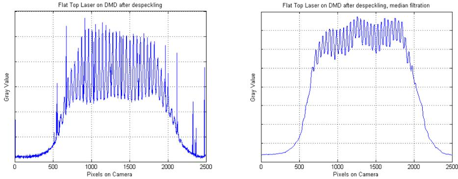
Figure 6 : Flat Top with rotating diffuser before (left) and after (right) median filtration
