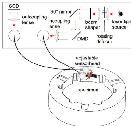
Figure 11 : Laser based endoscopic fringe projection system schematic
