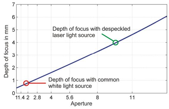
Figure 9 : Depth of focus in dependence of the Aperture respectively f-number
