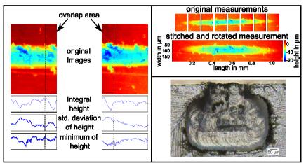
Figure 1: 1D-feature functions for overlap estimation (left), stitched microstructure (top right), profile image of undercut specimen (bottom right)
