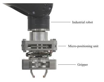
**Figure 1:** Industrial robotic manipulator augmented with high-precision micro-positioning unit and gripper for grasping optical components.
