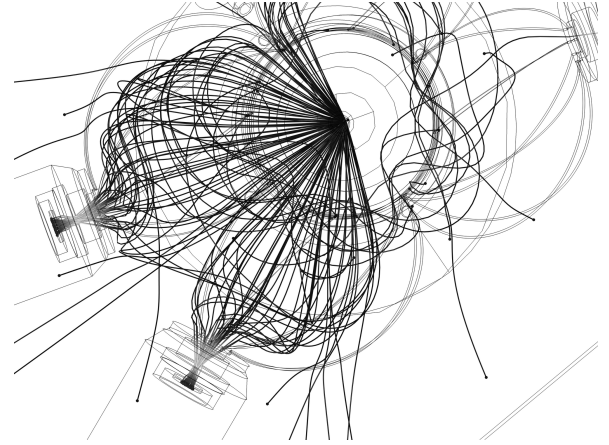
Figure 10: Top view on the simulation results for 120 electrons with cylinder: 38V, grid: -4V and gun shielding: -2V with 10 connection wires per detector on the left and 8 connection wires per detector on the right
