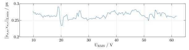
Figure 10: Minimum of the norm of the standard deviation of all reprojection errors for each focus adjustment
