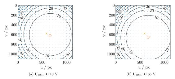
Figure 15: Visualization of the displacement due to radial distortion for two exemplary focus adjustments
