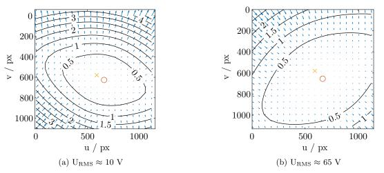
Figure 17: Visualization of the displacement due to tangential distortion for two exemplary focus adjustments
