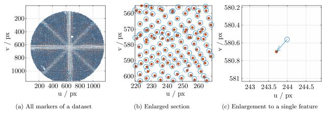
Figure 6: Reprojection error (blue arrow) of all calibrated features of an exemplary calibration dataset
