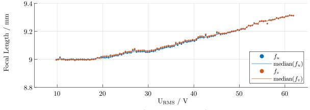
Figure 11: Intrinsical focal lengths (in world coordinates) for each focus adjustment
