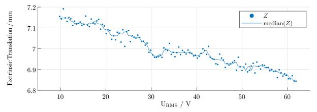
Figure 19: z component of the extrinsic translation for each focus adjustment
