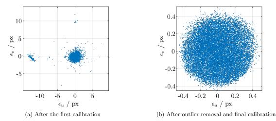
Figure 7: Location of the reprojection errors of all extracted features of an exemplary dataset
