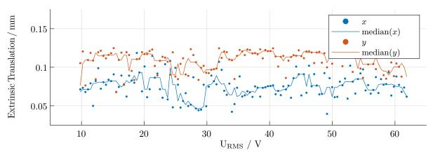
Figure 18: x and y components of the extrinsic translation for each focus adjustment
