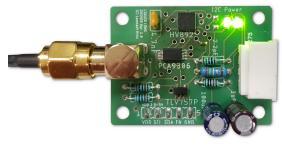
Figure 2: Driver board used for the generation of output levels
