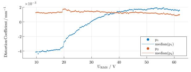
Figure 16: Coefficients of tangential distortion with respect to each focus adjustment
