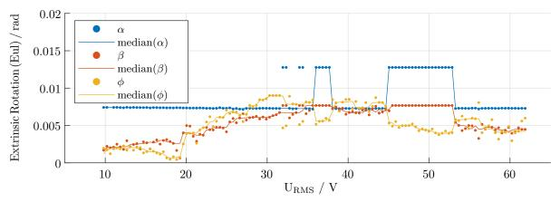
Figure 20: Representation (in Euler angles) of the extrinsic rotation for each focus adjustment
