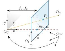
Figure 4: Overview of the pinhole camera model
