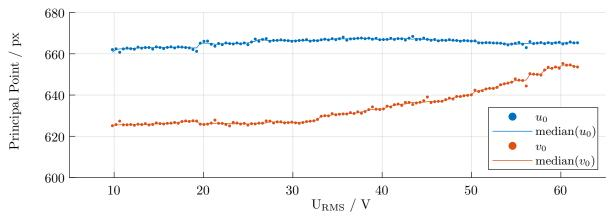
Figure 13: Coordinate of the principal point for each focus adjustment
