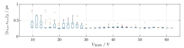
Figure 9: Boxplot of the euclidean norm of the standard deviation of all reprojection errors for each focus adjustment
