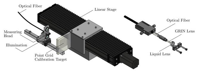
Figure 1: Experimental setup at the measuring head end with all essential components and optics
