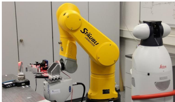
Fig. 5 Robot guided microscale fringe projection system
