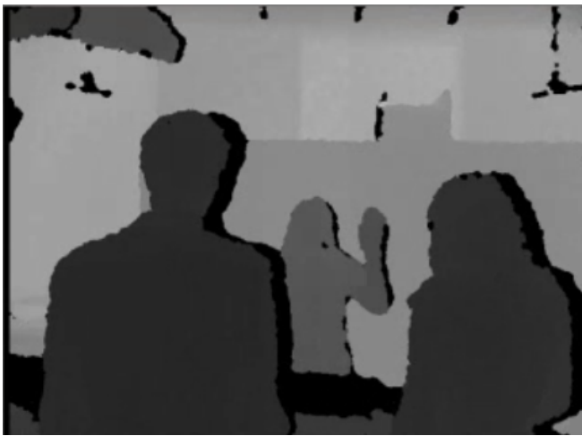
Fig. 10. Multiple people positioned between user and sensor system. Sensor viewpoint of the occluded user.
